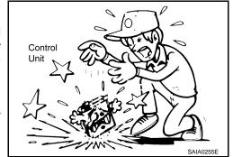
When using a DMM, be careful not to let test probes get close to each other to prevent the power transistor in the control unit from damaging battery voltage because of short circuiting.
