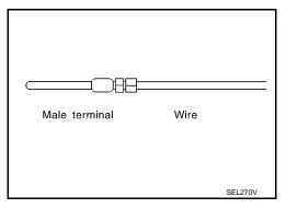
3. While holding the wire of the male terminal, try to insert the male terminal into the female terminal.
