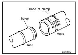
After installing plate clamps, apply force to them in the direction of the arrow, tightening rubber hose equally all around.
