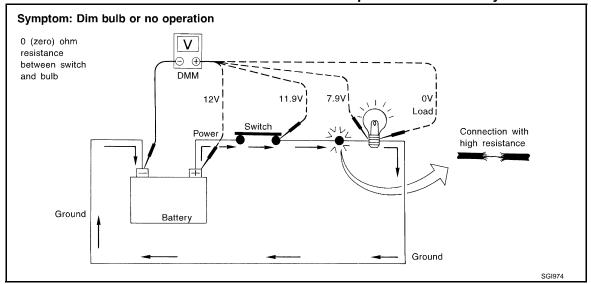
Measuring Voltage Drop — Steb-by-Step
