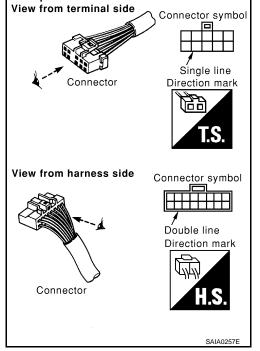
Male and female terminals Connector guides for male terminals are shown in black and female terminals in white in wiring diagrams.
